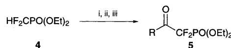
Scheme 1 Reagents and conditions: i, 1.0 equiv. LDA, CeCl 3 , THF, -78^\circ\text{C} ; ii, RCO 2 Et; iii, HCl(aq)
